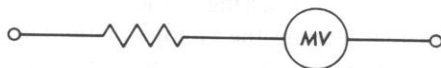
Figure 11-94. A series resistance and millivoltmeter combination make up the basic parts of a voltmeter.
